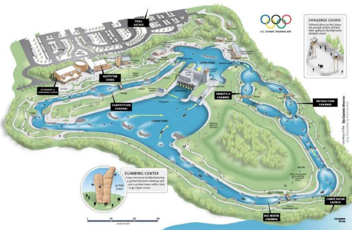
Figure 2: The US National Whitewater Center is a pumped whitewater park that pushes water from the bottom pond to the top where it then flows by the force of gravity through four channel segments.
